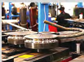
11 Axis Pipe Maneuvering
