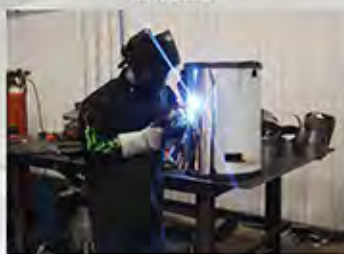
Welding Stainless Steel Housing
