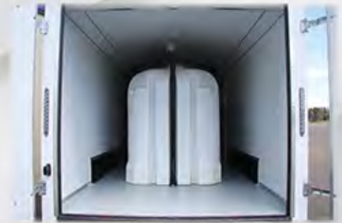
740 Gallon Water Tank (Back)
